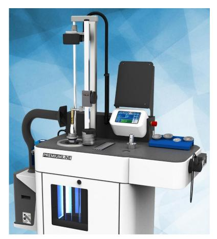
In order to ensure the longevity of the tool holder the system uses proven fixed parameters to shrink reliably. Optimum safety for the operator as no contact with the hot shrink fit chucks is necessary. Tool profile independent cooling with no need for adapters.
