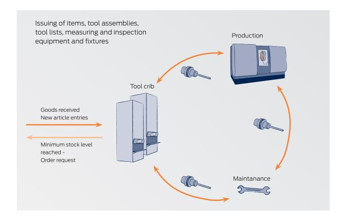
The TDM Tool Crib Module organizes items and tool assemblies according to stock level and tool crib location, taking the current location of the tool into account. This makes your tool organization transparent and efficient. The TDM Tool Crib Module allows you to create flexible tool crib structures, since it can manage both manual and automated storage systems.
